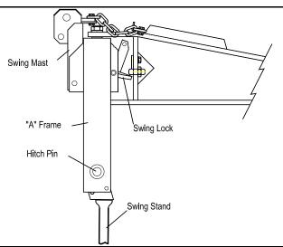
Figure 2. Swing Hitch Operation
